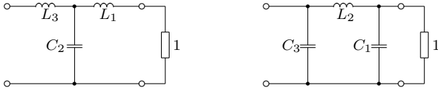
Fig. 2. Singly Terminated Third Order Lowpass Filters
